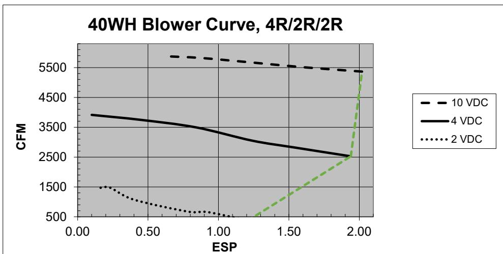
Note: Recommended range between 3400-3600 CFM. Could do lower if measures to prevent coil freezing are taken
