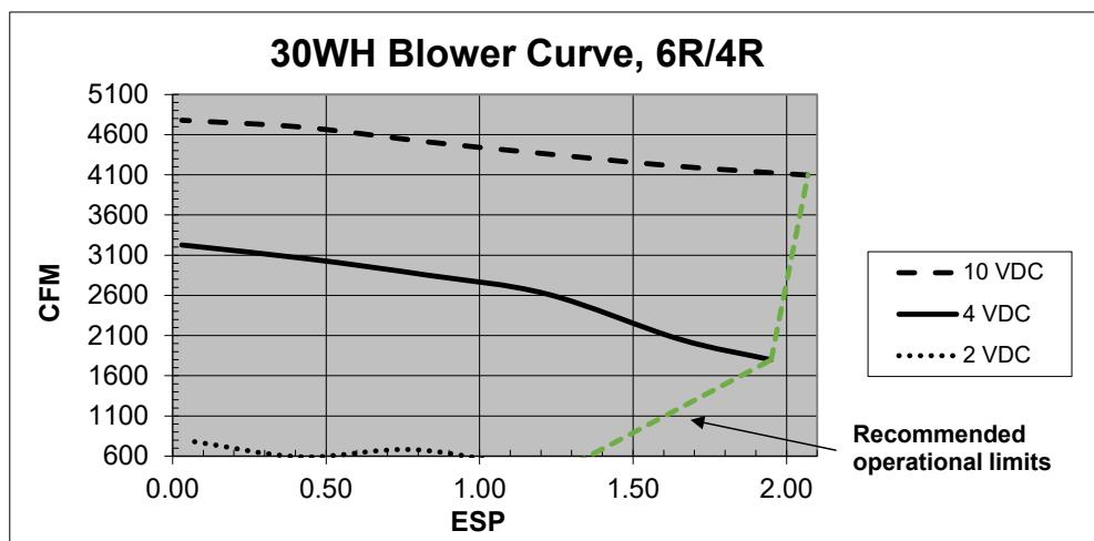
Note: Recommended range between 2500-3500 CFM. Could do lower if measures to prevent coil freezing are taken
