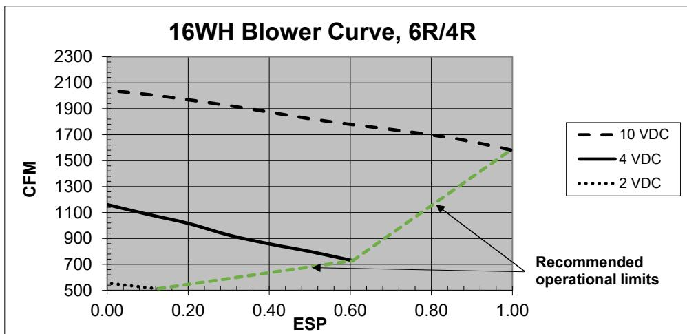
Note: Recommended range between 1400-1800 CFM. Could do lower if measures to prevent coil freezing are taken
