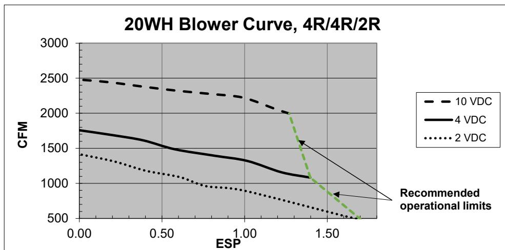
Note: Recommended range between 1800-2200 CFM. Could do lower if measures to prevent coil freezing are taken
