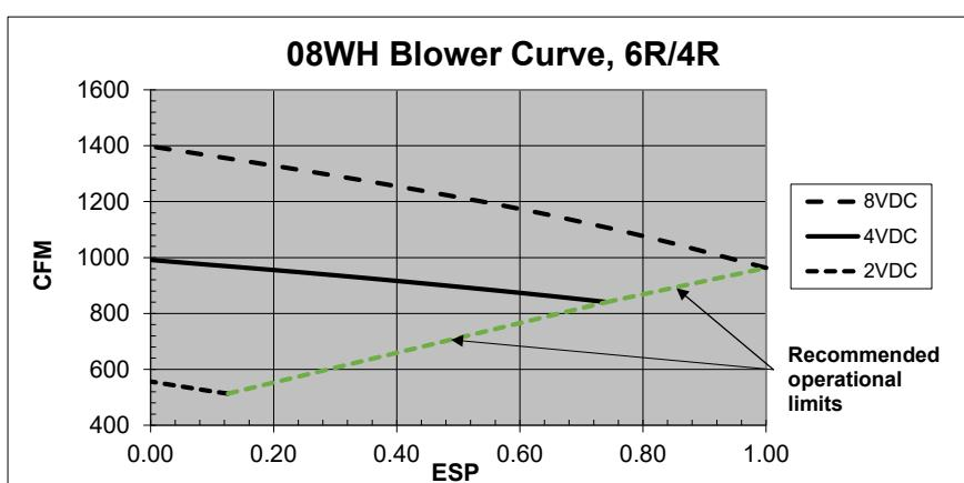
Note: Recommended range between 600-1000 CFM. Could do lower if measures to prevent coil freezing are taken
