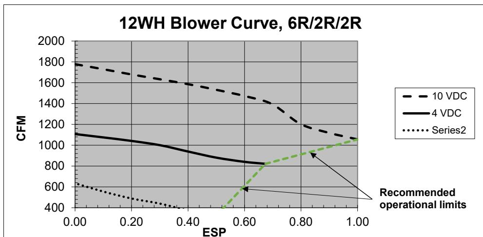
Note: Recommended range between 1000-1400 CFM. Could do lower if measures to prevent coil freezing are taken
