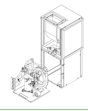
Commonly accessed items such as the TXV, refrigerant access ports and pressure switches are also accessible from the front of the unit without needing to remove the electrical box. For fast diagnostics, the unit also has a see through sight glass that allows the technician to read the control board status codes without removing the front panel.
