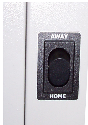
Optional Vacated Premises Selector Switch (Kit# 9WS01)
